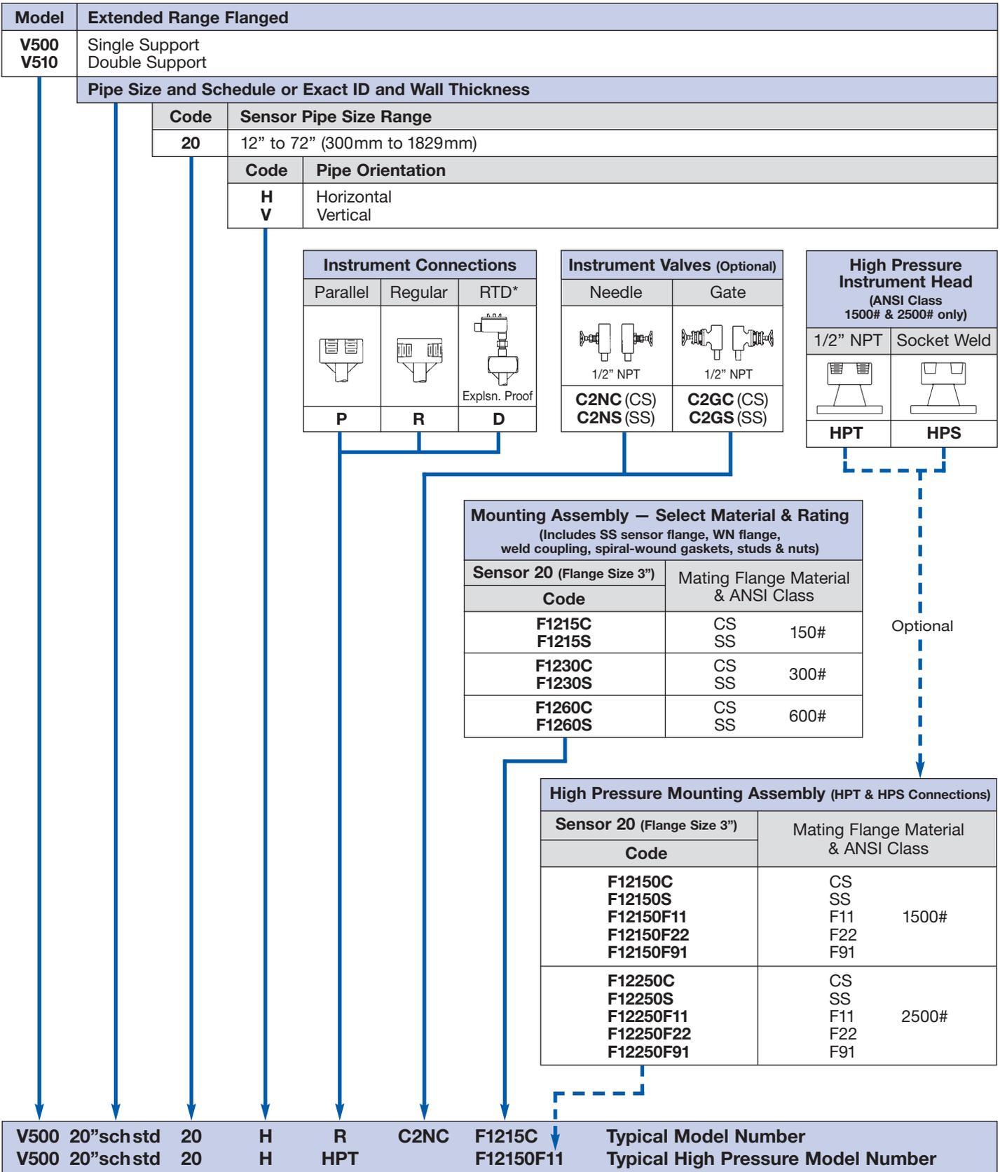
\* For high pressure (>500psig) or high temperature (>500°F), remote mount RTD in a thermowell is preferred.
